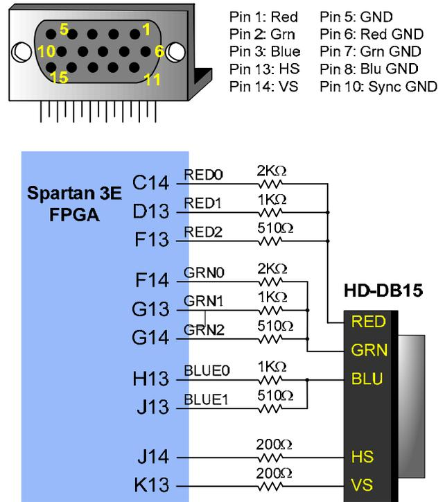
Figure 13. VGA pin definitions and Basys2 circuit
