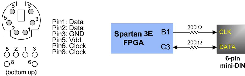
Figure 9. PS/2 connector and Basys2 PS/2 circuit
