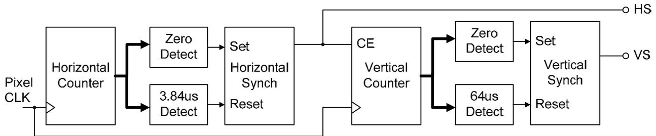
Figure 17. Schematic for a VGA controller circuit
